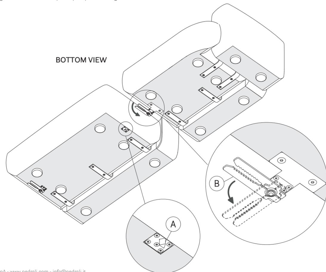
**EN** - Align and bring the modules closer together by pushing them firmly so that they are connected by means of the linking system (A) and (B). We recommend removing the serrated hook (B) when not in use.
